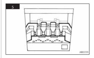
6.2 Locate the rear panel against the spacer brackets and slide down so that it locates on the ledge of the flame baffle, see diagram 6.
